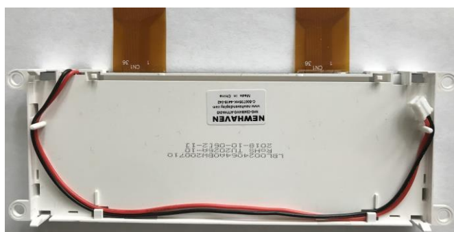
Figure 2-1: LCD Backlight Cable Routing
