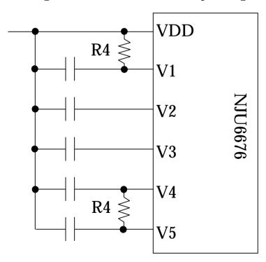
For reference:  $R4 = 68K\Omega \sim$  (by our testing R4 is from  $68K\Omega$  to  $150K\Omega$ )
